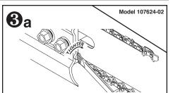
Turnchaintensioningscrewclockwise to tension saw chain or...
